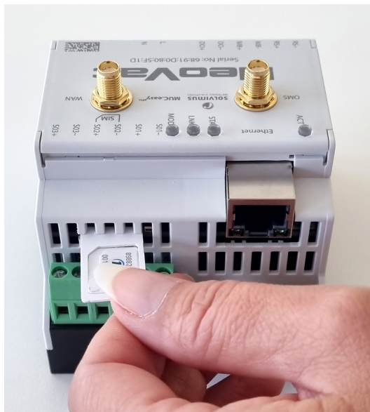
Figure 2: Insertion of the SIM card in a device with integrated mobile network modem
