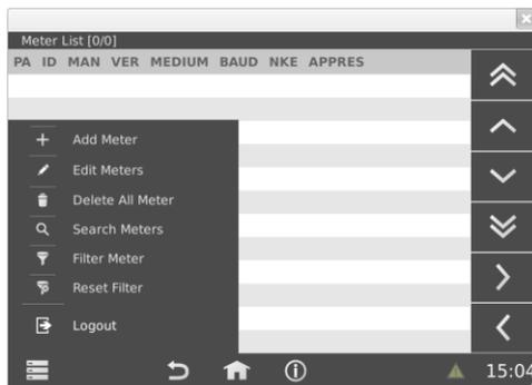
First you specify whether the search shall be done by primary or secondary addressing. There is a fast method and an intensive method with more retries and more tolerant timing (slowly but safer in case of wide M-Bus networks with many meters). If the installed M-Bus meters have not been programmed with a unique primary address, you must perform a search for secondary addresses.
