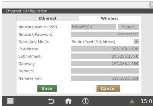
The “Wireless” configuration is similar to the “Ethernet” (RJ45) configuration. There is an additional search for WIFI networks followed by a selection of the WIFI access point (AP) and an input field for the password.
