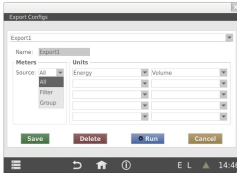
The most important values energy and volume are selected in the above example. There are further possibilities to choose the data of all meters (All) or meters from a predefined filter (Filter, e.g. all electricity meters) or meters from a specific group or tenant. The created export config can be saved under a name for further use with “Save”. The button “Run” starts the export immediately:
