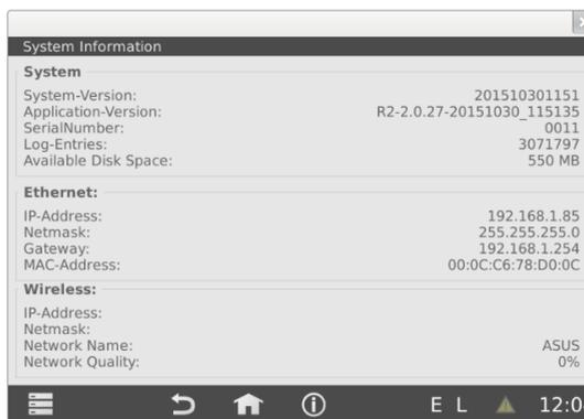
If the WebLog contains an optional WIFI module, the signal quality (0 to 100%) is shown in the wireless information area. A web browser can access the WebLog via network after the network configuration has been done correctly. From this point you can continue the configuration using a web browser (e.g. Firefox).
