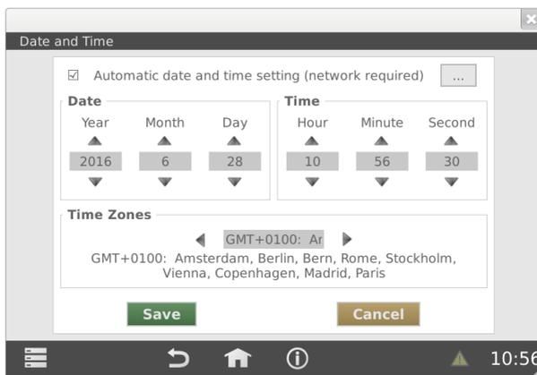
If the option “automatic date and time setting (network required)” is activated, the WebLog synchronizes the internal clock once per day with the clock of a time server in the Internet. By a click on the button with the three points you can change the predefined time server - for example if the device is operated in a local network with its own time server. The button “Save” stores the time settings.
