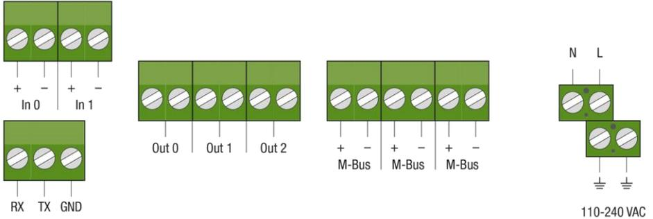
There are three equivalent two-pole pluggable screw terminals to connect the M-Bus. An electrician shall connect the main supply to the screw terminals on the right (110 to 240 VAC). Phase, neutral and earth (PE) are marked with L, N and earth symbol. The remaining pluggable terminals are reserved for future extensions.
