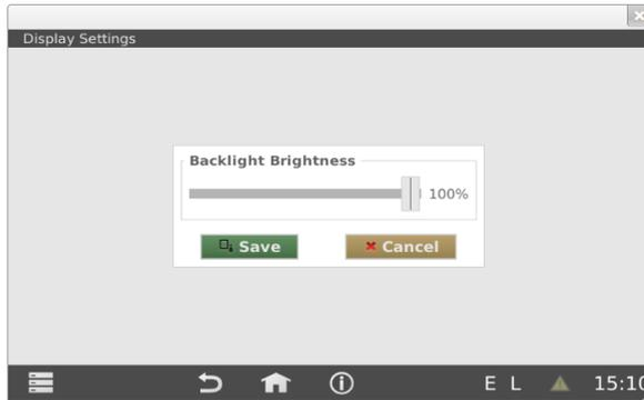
“Save” stores and activates the new backlight brightness. “Cancel” withdraws the changes and restores the former setting
