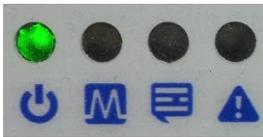
Four LED's on the front side of the WebLog show status information about the power supply of the CPU and important system events.
