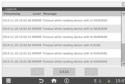
The entries in the log book can show for example errors occurred during communication in M-Bus. The above example shows a meter which could not be read several times during logging. A short circuit on the M-Bus is also a possible error message. Another example of possible error messages is that the device could notify a failed synchronisation of the clock from a time server in the internet.
