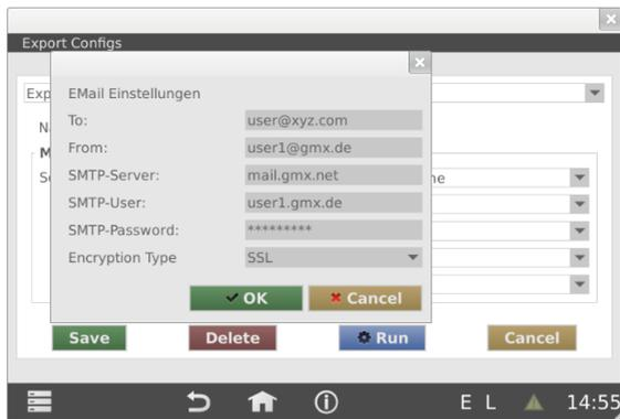
You have to enter the destination e-mail address and the SMTP server in case of an e-mail transfer. If you want to use your internal Microsoft exchange server, please enter the IP address of that server and the exchange user with password. The encryption type for MS Exchange is "Plain" (unencrypted). The example shows the settings for a GMX account using the GMX SMTP server. The e-mail sending with GMX needs encryption (Encryption Type = "SSL").
